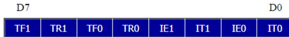
TCON (Timer/Counter) Register (Bit-addressable)
